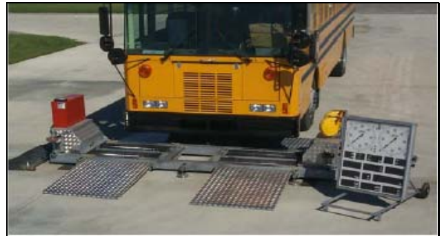
Figure 11. Category M 3 vehicle during roller brake test
