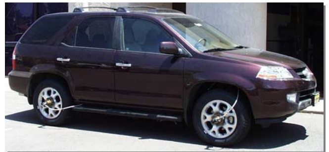
Figure 1. Vehicle instrumented for FMVSS 135
