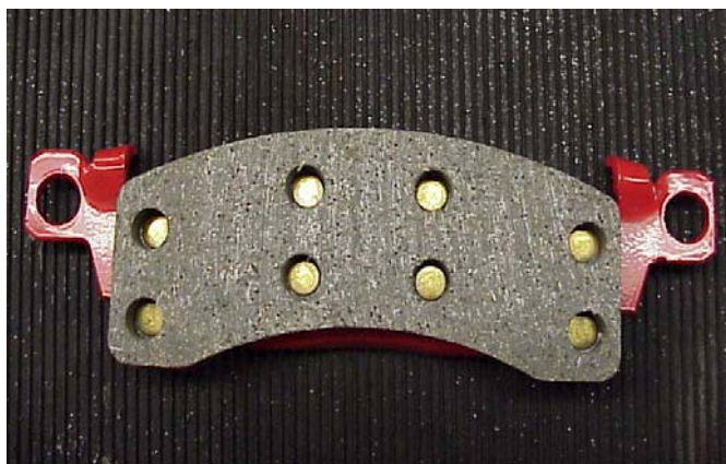
Figure 1. Brake Pad Used for Testing
